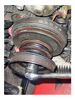
**While still holding cam bolt with wrench**, tighten clamp ring bolts. Remove 32V'r.
