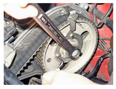
For advancing, or clockwise adjustment, slide indicator into the hole that corresponds to the amount of advance desired, with crankshaft at #1 TDC.
