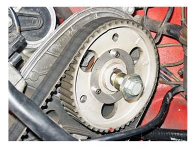
Reinstall cam bolt with spacer.
