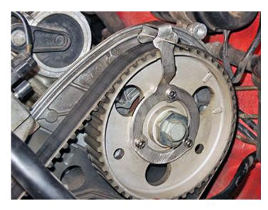
Insert needle into hole that most closely fits into the housing indentation **V**.
