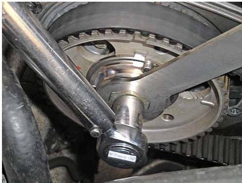
**Torque cam bolt to 47 ft. lbs. (65 Nm) with torque wrench.**
