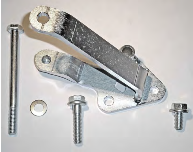
Left: optional air pump accessory bracket and hardware.
