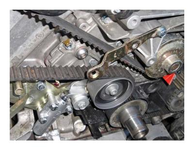
Install ground terminal on water pump. 7 ftlbs
