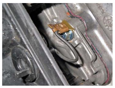
After installing center cover, plug sensor wire onto ground terminal.
